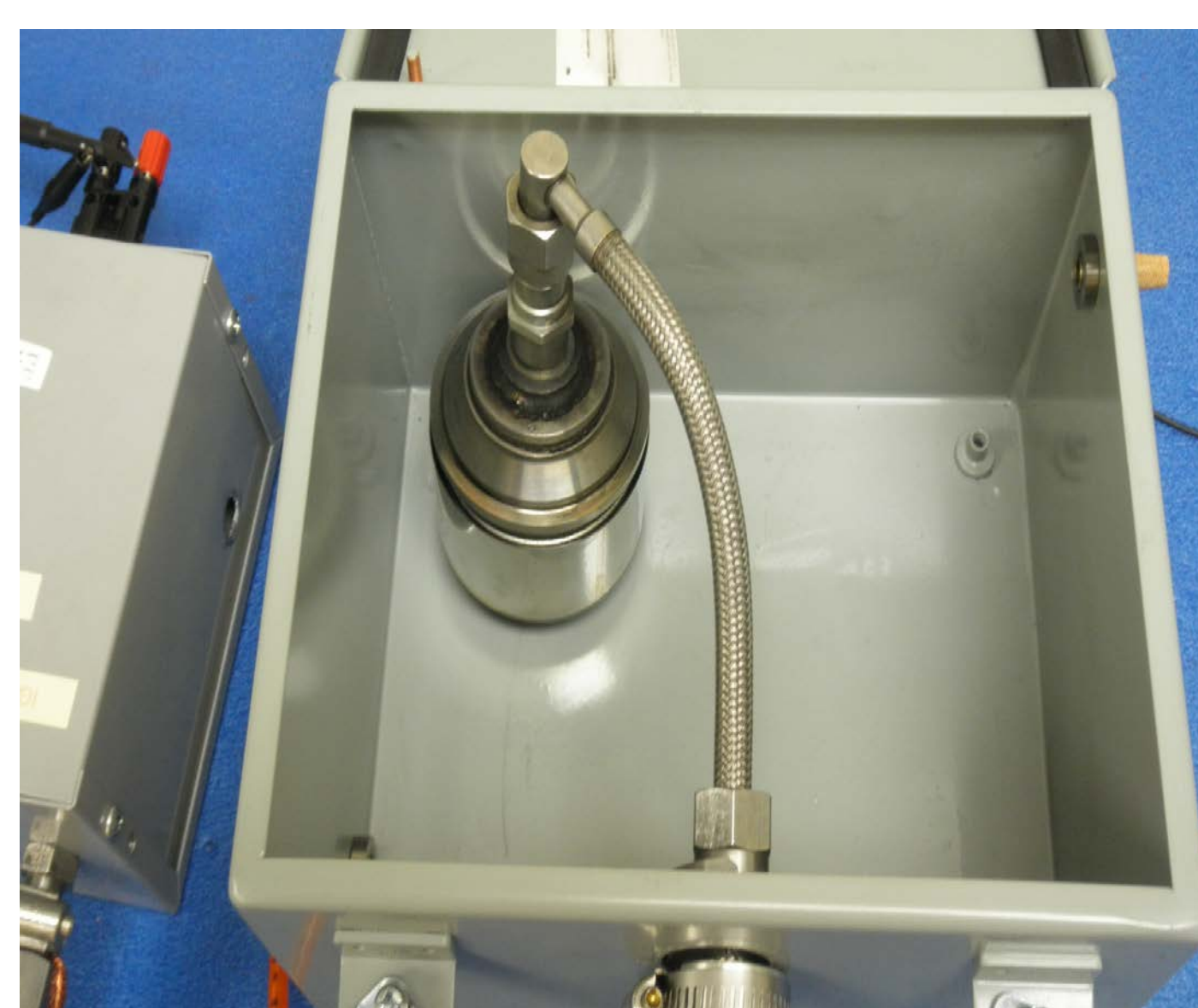
Figure 4. Wet Spark Test - Apparatus, Inside View
