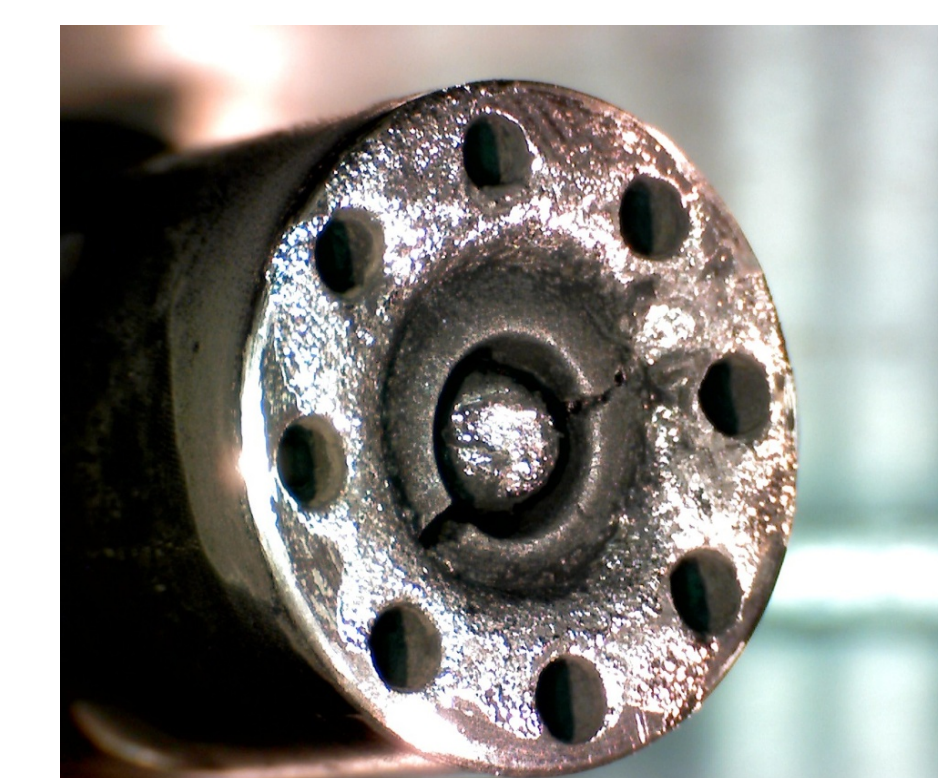
Figure 7. Alloy Wet Spark Test – End of Test
