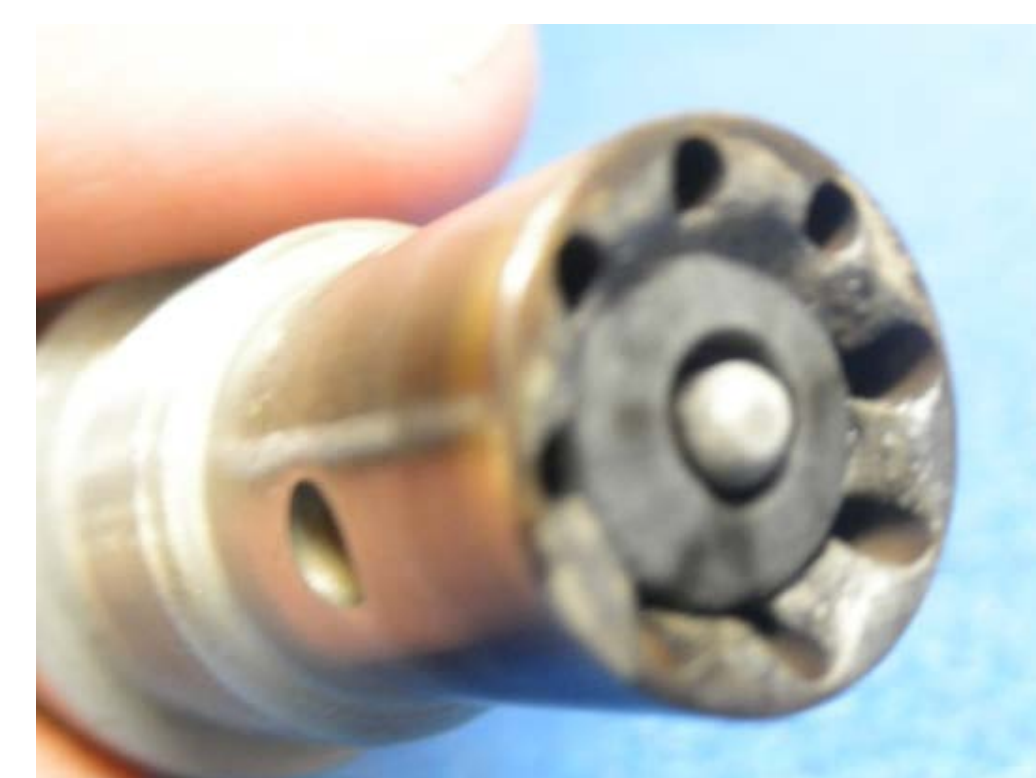
Figure 6. Dry Spark Tip – End of Test
